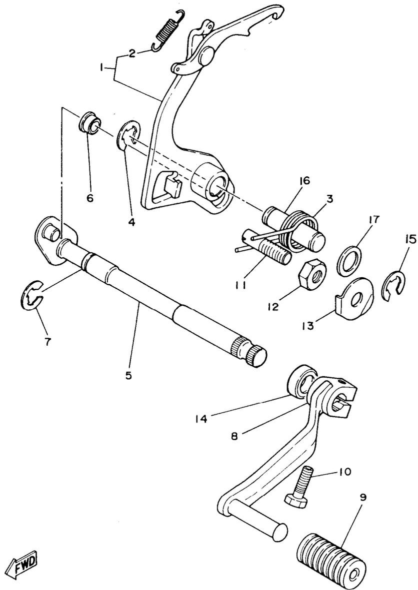
FIG. 14 – EIXO E PEDAL DE CÂMBIO
